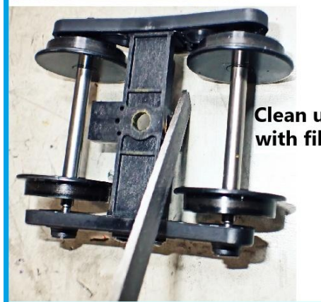
Example razor saw to cut off tang
